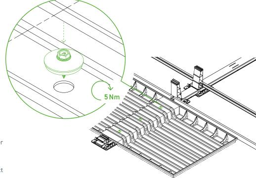
Place the ballast tray between the tower and the base centrally on the exact positions. Exact positions of the ballast trays can be found in the current project report. Then screw each ballast tray centrally and evenly distributed on the main bottom profile by means of the supplied drilling screws (three pieces). Observe the maximum torque of 5 Nm!
