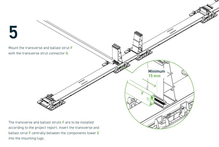
If no cross strut connector  ${\bf G}$  is installed, fix the cross strut and ballast strut  ${\bf F}$  to the tower  ${\bf E}$  with one M8 x 30 screw each.
