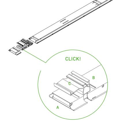
The base **C** is to be pushed into the main bottom profile **B** until the click lock engages with an audible noise. Two bases must be installed per main bottom profile. At the beginning and end of a main bottom strand, a starting and end bottom profile **A** must also be clicked onto the base **C**.
