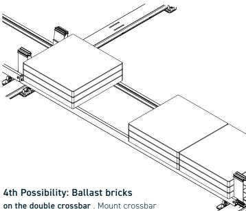
on the double crossbar. Mount crossbar and ballast strut on both sides of the tower as described in step 5, place ballast bricks evenly distributed on the crossbars near the tractor.
