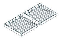
Remove gravel/substrate fill up to the inner edges of the main bottom profiles in the area between base and tower. The depth of the excavation should be at least 50 mm from the top edge of the bed, in order to ensure that the ballast trough rests flat on the remaining bed or the roof surface. When placing the ballast tray directly on the roof covering, care must be taken to ensure a clean surface in order to avoid long-term damage.
