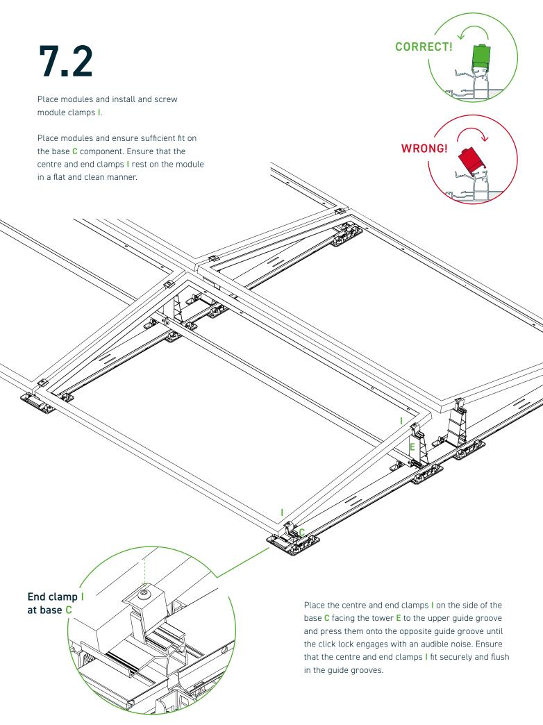
7.3 Tighten the terminal screws. The installation instructions of the module manufacturers must be observed. Middle clamp | Observe tightening torque of 10 Nm. Minimum 20 mm 10 Nm End clamp I CLICK! **DONE WITH THE BASIC SYSTEM!**
