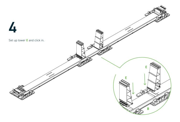
Press the two central components tower  ${\bf E}$  with the detents pointing towards the centre of the rail, vertically into the two narrow recesses of the main bottom profile  ${\bf B}$  and push them towards the centre of the rail until the click detent clicks into place with an audible noise.
