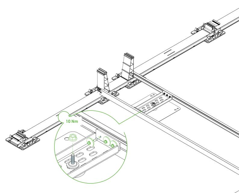
To attach the connection point to the system, three supplied drilling screws are screwed into the transverse and ballast struts on each side through the USO sheet. The location and position of the USO connection can be found in the current project documents.
