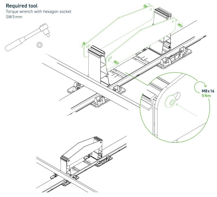
OPTIONAL ASSEMBLY STEP IRRADIATION SENSOR BRACKET
